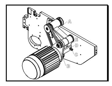
Dismount the rear machine covering and release the fixing nut D. By help of a forcing-off screw (C) between motor holder (B) and spindle body (E) you can change the inter-pulleys distance and so tighten the belts (A). When you push by hand to a middle of a properly tight V-belt by a force of 20 N (2 kg) - it should sag of nearby 10 mm. After tightening it is needy to tighten the fixing nut again and to mount the machine rear covering.
