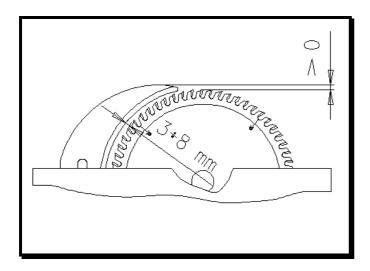
The riving knife prevents eventual workpiece enclosure behind the saw disk and its claps during sawing. This could come about a back cling. The riving knife must be mounted permanently. It is adjusted by scrolling so that its horizontal distance from the saw disk should be 3-8 mm and vertically 2 - 3 mm.
