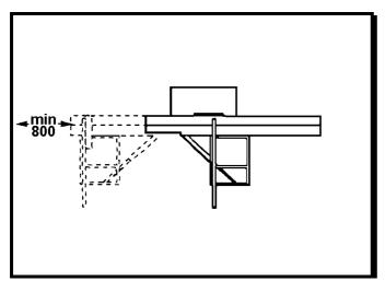
It is important to keep a free space of at least 0,8 m, requested as working space surrounding the machine. If a long peace is planed, it is necessary to have a sufficient space in front of and behind the machine in places of material in - and output.
