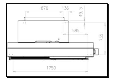
If you are sure that the placing of the machine is good, level the machine by help of forcing-off screws in machine feet. Use steel washers (part of delivery) under levelling screws and balance the machine in a plane with the clearance limit 1 mm/1metre and screw down machine feet into the bottom (anchor the machine).
