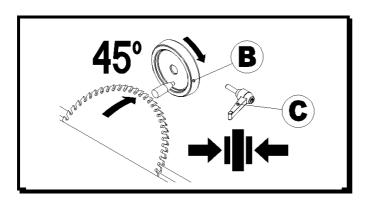
Height of the main saw blade is adjustable by the hand wheel (A) with the arresting screw clockwise = blade height + anticlockwise = blade height -The height of cut gets always adjusted "from below" that enables to adjust eventual allowance. The cut height is usually set so that
