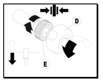
The height of scoring saw blade is adjustable by help of a screw with a hand star (D) and with the arresting nut (E). After releasing of the arresting nut (E) - the scorer lifts up when turning the hand star (D) with the screw to the right and vice versa. Tighten up the arresting nut (E) after setting the required height of the scorer.
