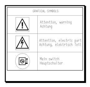
Informative shields and shields warning against dangers are placed at the machine frame.
