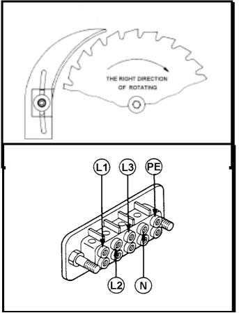
When standing at the place of machine operator - the main saw blade must rotate clockwise (= to the right), and the scoring saw blade, if installed, must rotate anti-clockwise (= to the left).
