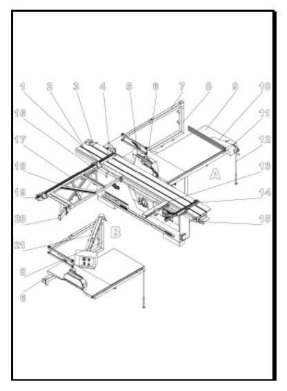
Mount supporting frame 19 onto sliding table 2, secure it with clips 1 against unhooking on both sides and with arresting accenter 16 against shifting; frame must be spared with a supporting arm 20
